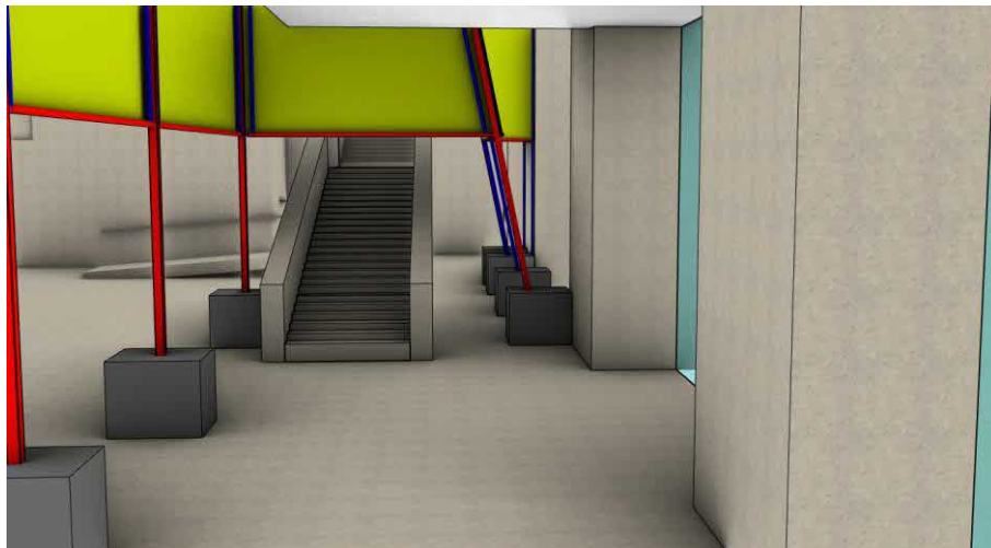
Figure 12: Ground floor West emergency exit. Kentledge to the moved away for the façade to free emergency access route.
